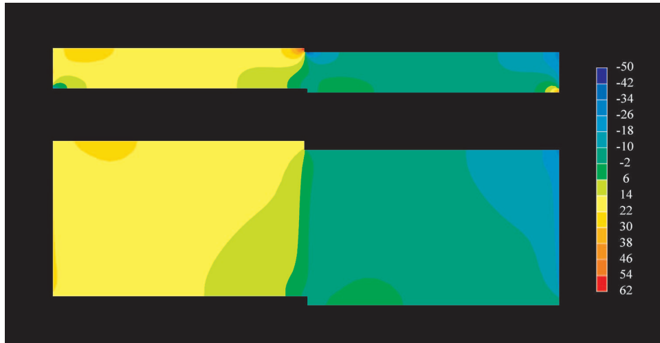
Fig. 4 Pressure (Pa) distribution for Re=500
